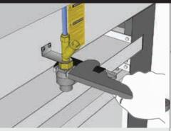
1. RESET WATER BLOCK: If a failure occurs causing a continuous water leak, the Water Block will shut off.
