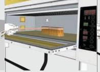
3. Clean Stone Brush and scrape out bake deposit or soot regularly during the day. Use a metal and soft brush!
