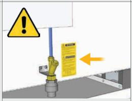
Read carefully the instructions on the label attached to the steam system
