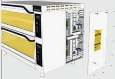
6. If possible, position the oven with easy access to the right hand panel to facilitate the electrical installation and future services
