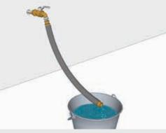
2. Open the water supply and let water run, this will clean the hose and any other residue in the water system before connecting the water supply to the Steam System
