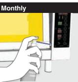
7. Lubricate Lubricate all the door bushings.
