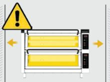
For ventilation of the oven, a space of at least 50 mm is needed between the oven and any adjacent wall, on all sides.
